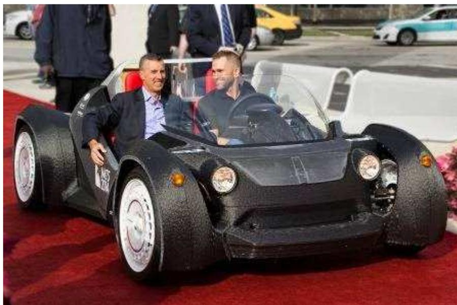
Figura 20 – Strati – Primeiro carro impresso em 3D. Fonte: <http://www.embedded-computing.com/embedded-computing-design/3d-printing-car-parts-is-a-potential-boon-to-auto-industry>
