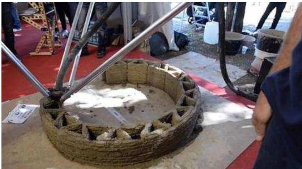
*Figura 24 - Projeto Wasp imprime casas. Fonte: <https://makezine.com/2014/10/14/wasps-20-foot-tall-3d-printer-to-make-mud-houses-in-rural-areas/>*
