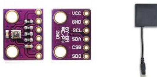
**Figura 4:** Barômetro BMP280 e HWS S-BPA-CM10.
