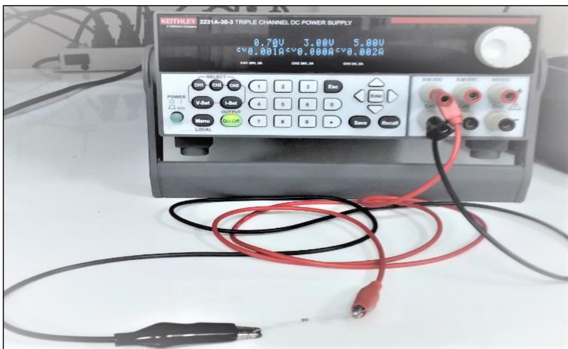
Figura 17 - DC Regulated Power Supply digital kethley 2231A – 30-3 Fonte: (Autor)
