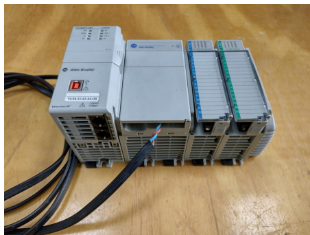
Figura 24 – CLP CompactLogix L30ERM.
